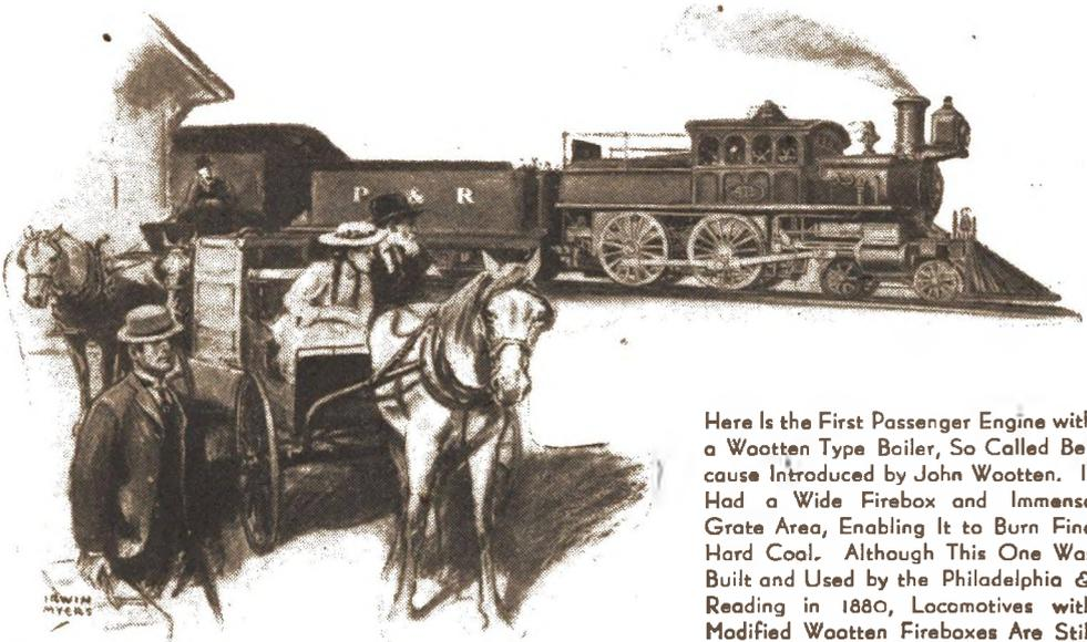
Here is the First Passenger Engine with a Wootten Type Boiler, So Called Because Introduced by John Wootten. It Had a Wide Firebox and Immense Grate Area, Enabling It to Burn Fine Hard Coal. Although This One Was Built and Used by the Philadelphia & Reading in 1880, Locomotives with Modified Wootten Fireboxes Are Still Standard on Many Roads
